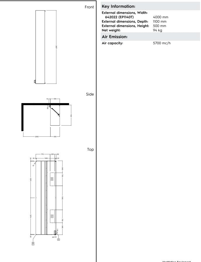
Ventilation Equipment 304 S/S Wall Hood+Filters 4000X1100mm
